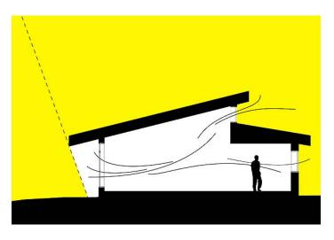
The firm performs precise shadow studies on their proposed designs so that they can size roof overhangs and shading devices accurately. While the science of passive solar design is not particularly complex, accuracy is important, otherwise the energy performance of the house may suffer. With Revit<sup>®</sup> they can be confident that the passive solar design strategies work prior to construction.
